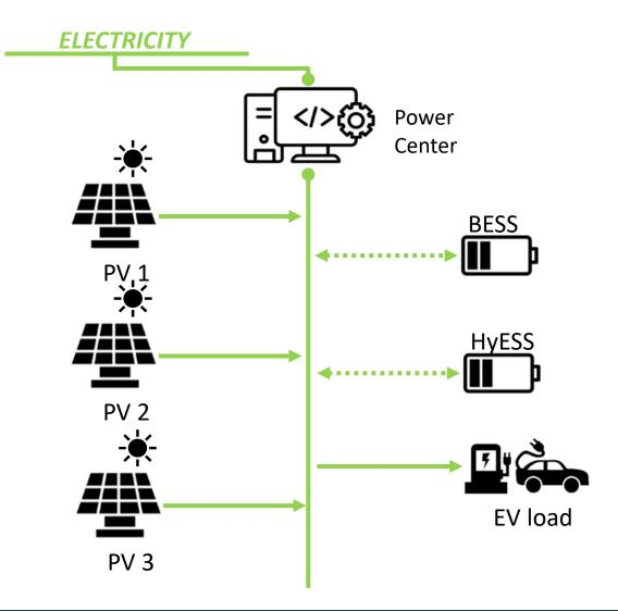
Power System (PV + BESS) connected to the National Electricity Grid through a single connection point
